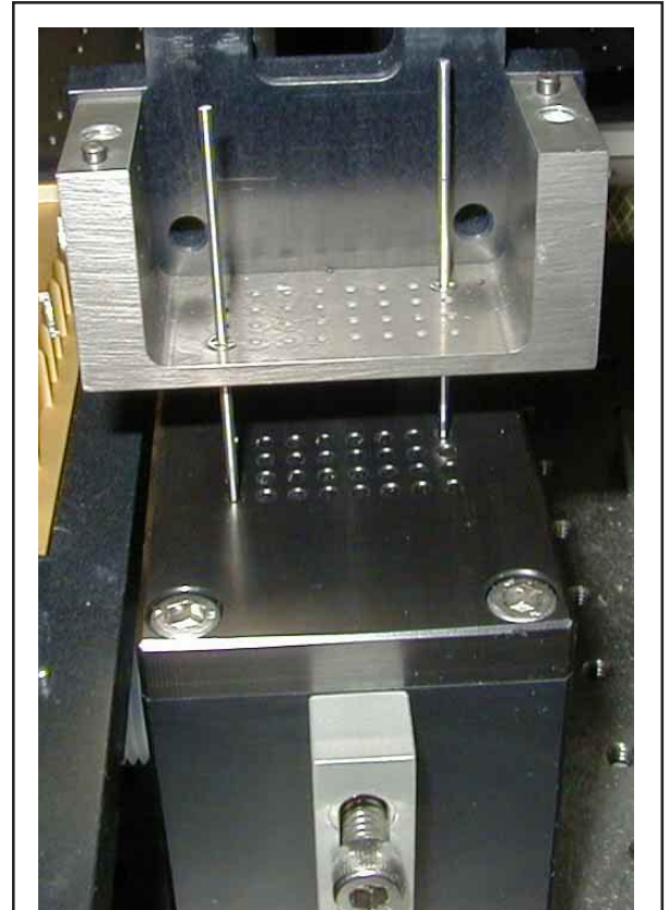
Use pins in the holder to properly align the dry station
