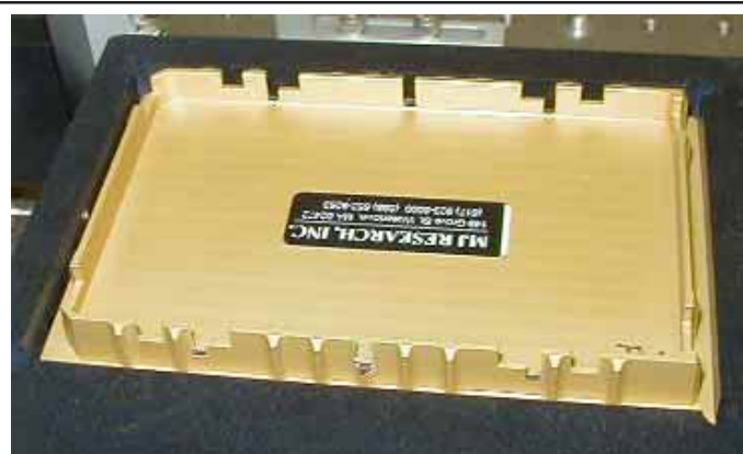
The MJ Research Plate Holder. Extra slots were cut to accommodate different 384 plates.
